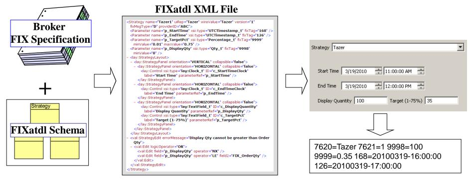
Broker creates a FIXatdl XML file describing its algorithms, parameters, FIX tag mappings, validation rules, and how the algorithms should be rendered in any 3rd party application OMS vendors parse these FIXatdI XML files & render them in their application eliminating the need for custom programming
